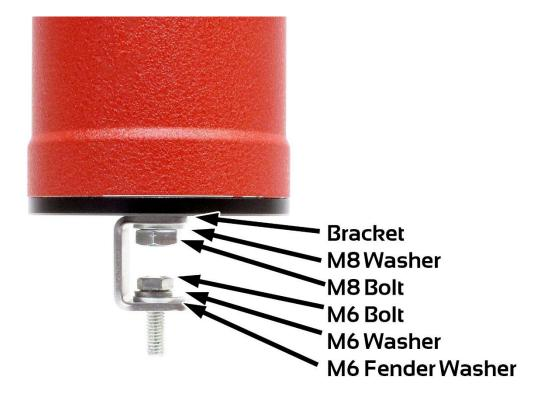
3. Place tank and bracket over hole in chassis, and install M6 bolt with small washer and large fender washer through bracket into chassis. Rotate tank to desired position, then tighten both M8 and M6 bolts to secure tank to chassis. **NOTE: Above picture shows how bracket is mounted to frame rail with coolant tank removed only for visual purposes. If you choose, you can mount bracket first, then tank to bracket.**
