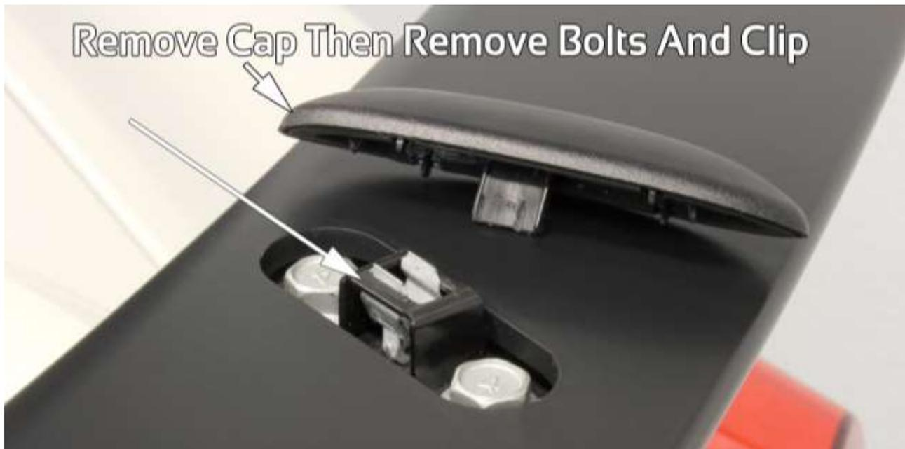
2. Remove bolts along with steel retaining clips from top of wing. **NOTE: Wing will be loose and could fall off car, take care not to bump wing while there are no bolts holding it to trunk.**
