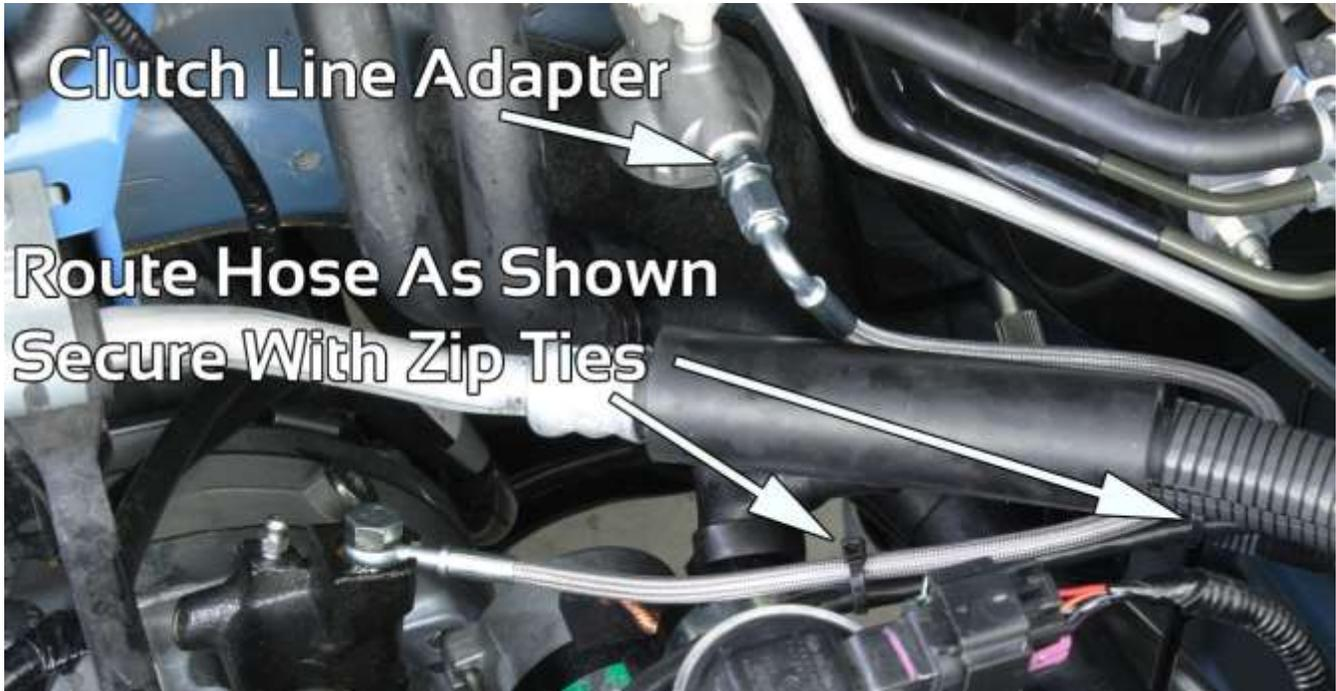
5. Loosen fittings and adjust so hose routes as shown in picture. Tighten all fittings down and secure with supplied zip ties.
