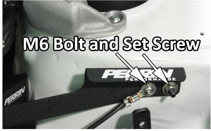
11. Install PERRIN Master Cylinder support bracket (black aluminum part) to PERRIN Master Cylinder brace using (2) supplied M6x10 button head screws and (2) M6 flat washers. Leave bolts slightly loose for now.
