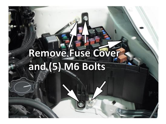
3. Pull fuse box forward in car roughly 5" to expose shock tower, fuel lines, EVAP dampener (If equiped), and fuel line bracket.
