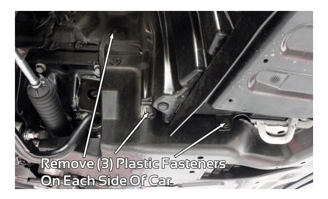
3. Using proper panel removal tool or flat head screwdriver, locate and remove (11) plastic fasteners and (2) 12mm headed bolts from lower portion of splash guard as shown below.
