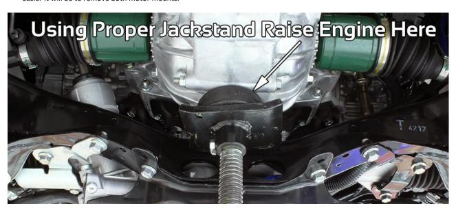
11. Using a 14mm socket and a universal joint, locate and loosen (2) M10mm bolts securing front portion OEM motor mounts to engine. These are located between the subframe and header as shown below. **NOTE: These are not removed to make next step easier.**
