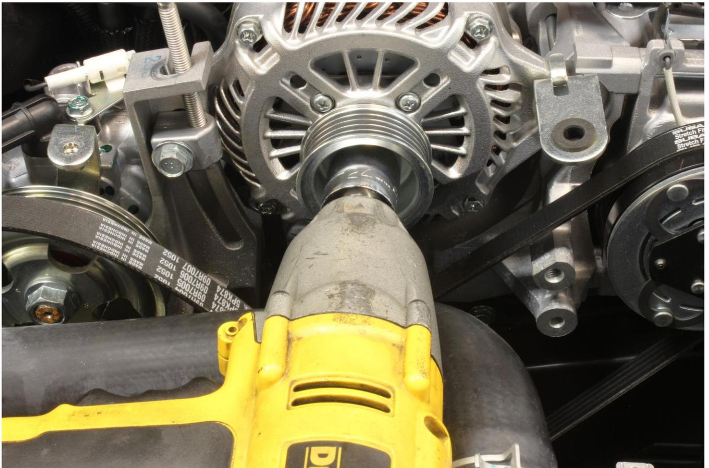
4. Lift alternator up to allow an impact gun with the 24mm socket to fit over nut. Unscrew nut (standard counterclockwise direction) from alternator. **NOTE: This may take several short bursts (with the pulley stopped between bursts) to free pulley from alternator. DO NOT install something through the insides of the alternator while trying to remove pulley.**
