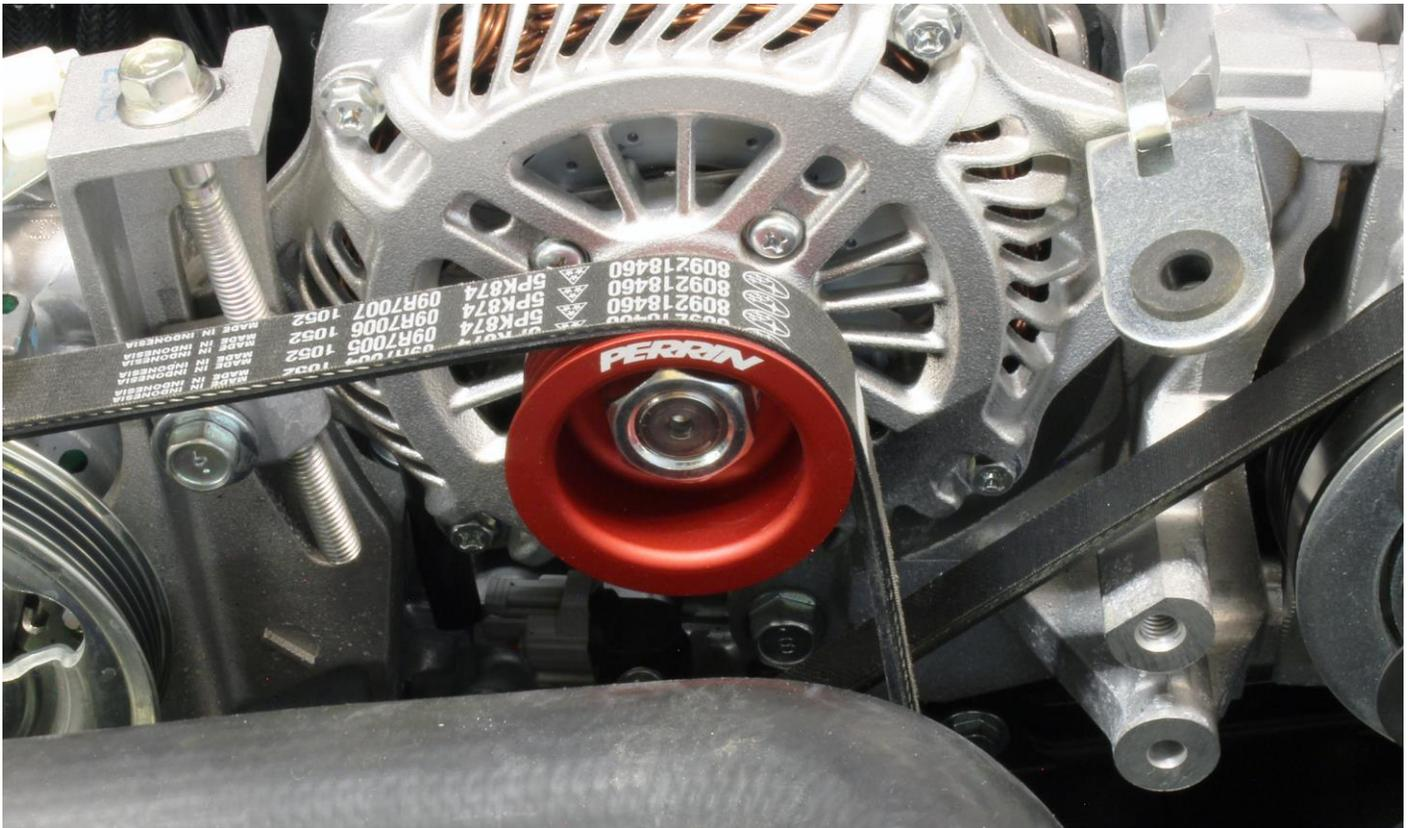
2. Lift alternator up to allow impact gun and socket to fit over nut. Tighten nut on pulley using short bursts from the impact gun until you see the nut stop spinning.
