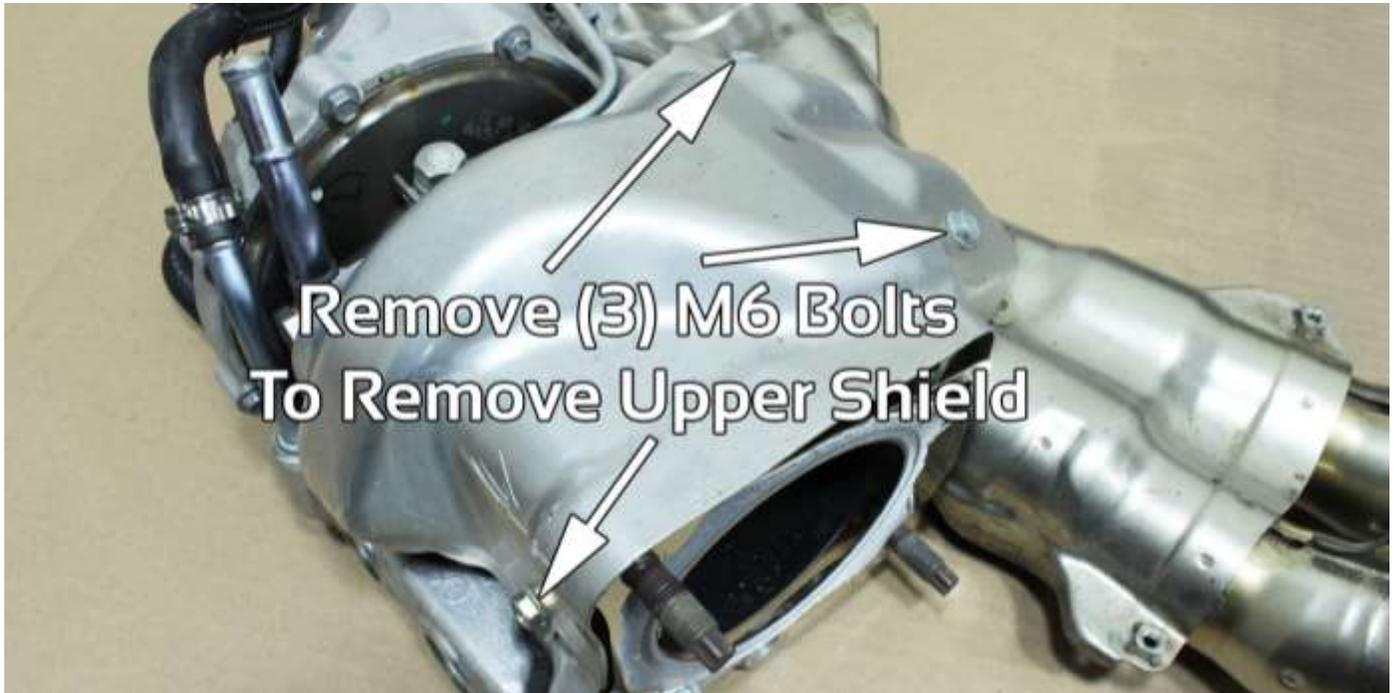
18. Flip header and turbo over, then remove (4) M6 bolts securing header heat shield to header. Remove both upper and lower shields from header. These will NOT be reused.
