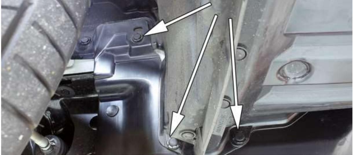
3. Using proper panel removal tool or flat head screw driver, locate and remove (7) plastic fasteners and (2) 12mm headed bolts from lower portion of splash guard. See picture below.
