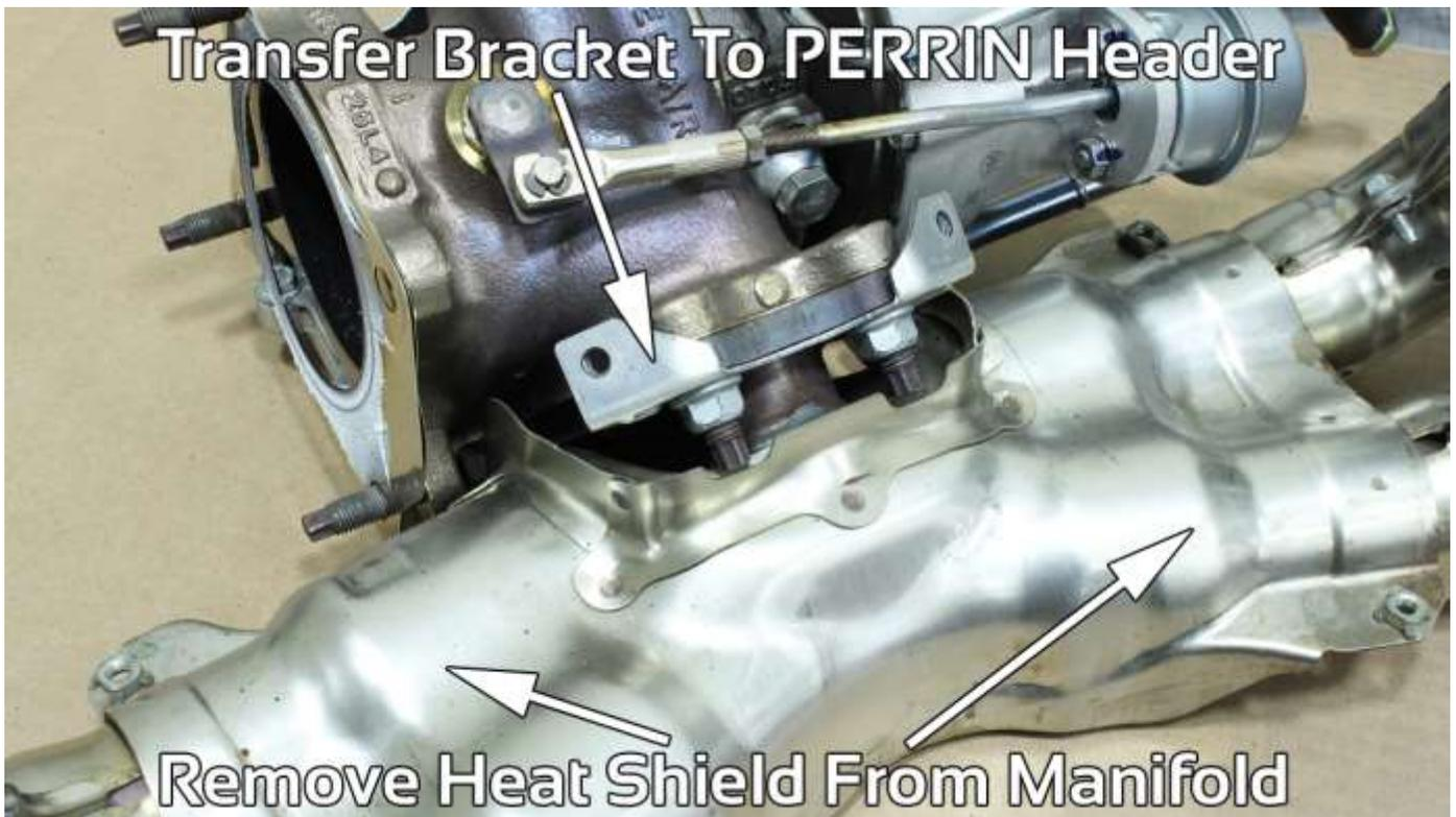
20. Install new OEM gasket onto turbo and place PERRIN header over studs. Place heat shield bracket on upper studs as shown, apply supplied Anit-seize compound to thread, then secure with OEM nuts removed. Tighten nuts to 40ft-lbs.
