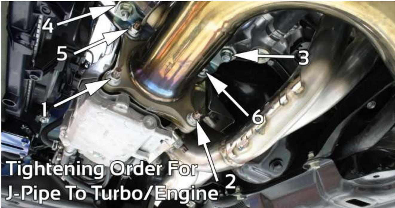
27. Loosen (2) M8 bolts securing upper turbo support bracket at engine, then re-tighten to 15ft-lbs. **NOTE: This step is important to relieve any unwanted pressure on the PERRIN header.** In the same order as in the above step, fully tighten bolts and nuts to 31ft-lbs. **NOTE: Not using the OEM turbo/header support brackets will cause the header to fail and will void the warranty on your PERRIN Header.**
