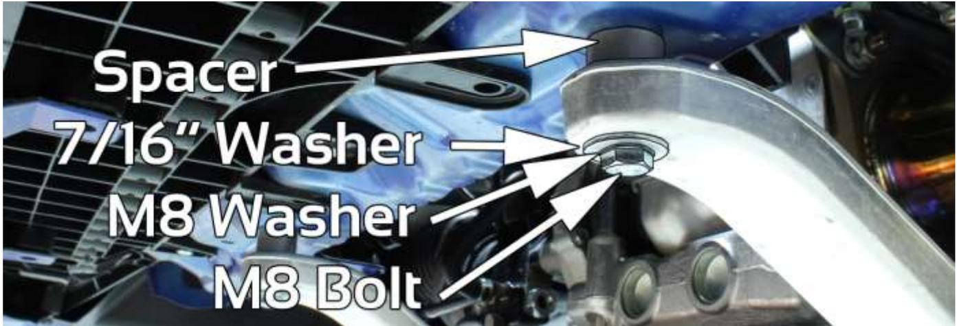
40. Reinstall OEM skid plate making sure to place supplied spacers between it and the chassis. Use supplied M8x55 bolts, M8 fender washers, and 7/16" flat washers to secure skid plate to chassis. Tighten bolts to 15ft-lbs.
