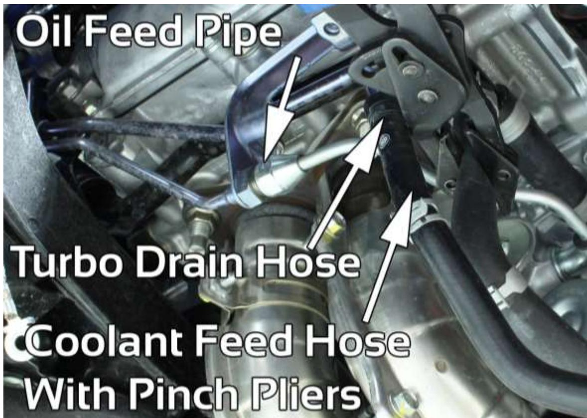
12. Disconnect turbo oil feed pipe using two open ended wrenches. **NOTE: Never use one wrench to tighten!**
