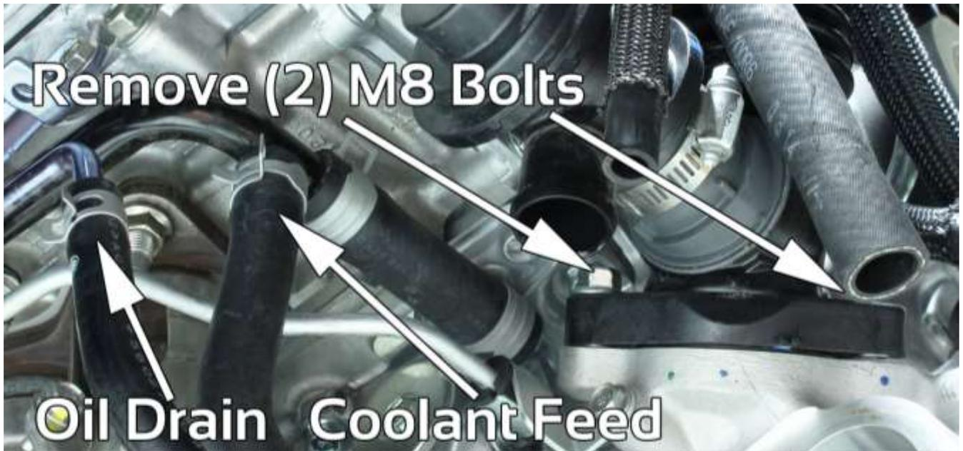
11. Removed (2) M8 bolts securing plastic boost tube to turbocharger (shown above). **Note: Rear most bolt is difficult to reach and best to use a gear wrench to remove.**
