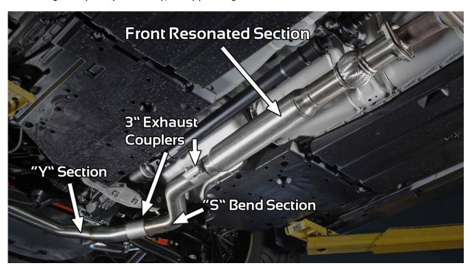
8. Adjust both 3" exhaust couplers so they are equally covering both tubes. Then rotate so the bolts can be easily reached and do not hang down below the car. Snug down hardware to hold tubes in place.
