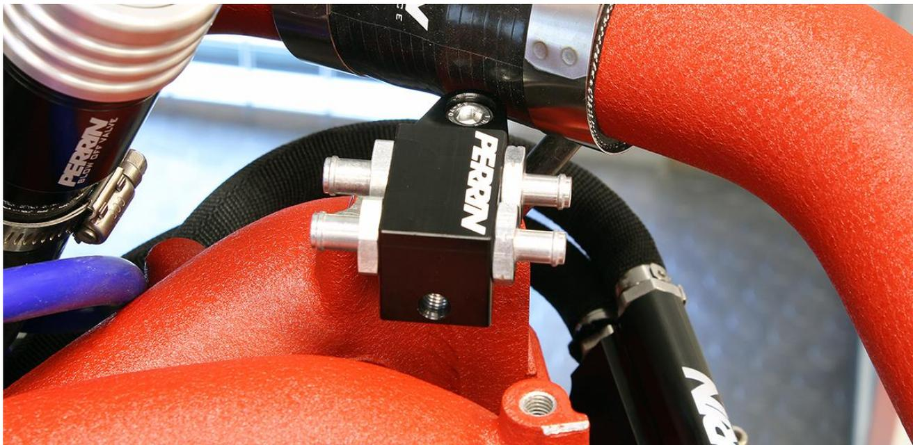
Threaded hole on side of junction block is used to hang the 04-05 STI fuel pressure regulator from.
