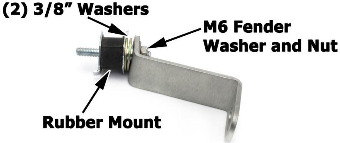
9. Install supplied bracket (with rubber mount) to threaded hole in frame rail and secure using supplied M6 screw and fender washer. Leave loose until air intake pipe is mounted.
