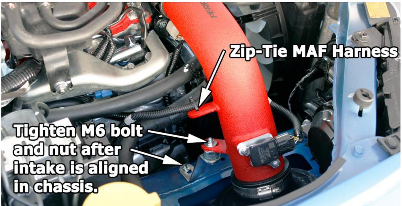
19. Re-install plug/harness to MAF sensor making sure that small tab locks into place.
