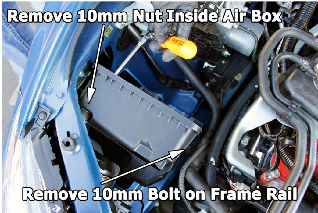
6. Remove front section of air box from vehicle.
