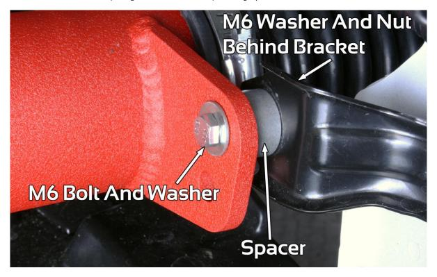
15. Using the next two pictures for reference, locate hole in chassis just below the headlight as shown below. Install supplied bracket (slot side up) with spacer to hole on chassis and secure with supplied M8 screw, washers and nut. Leave hardware loose at this time.
