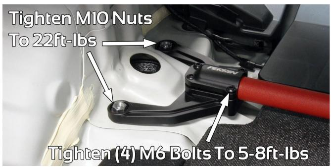
Trunk liner is removed in picture to better show the top of the shock tower
