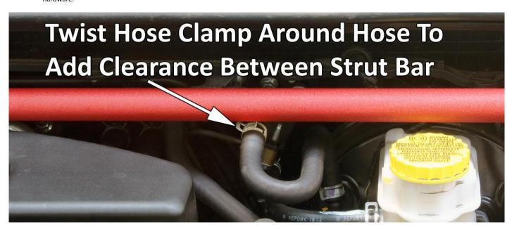
8) For non-turbo models, add clearance between strut bar and brake booster hose by either rotating hose clamp down or pushing down on piping to bend it out of the way.
