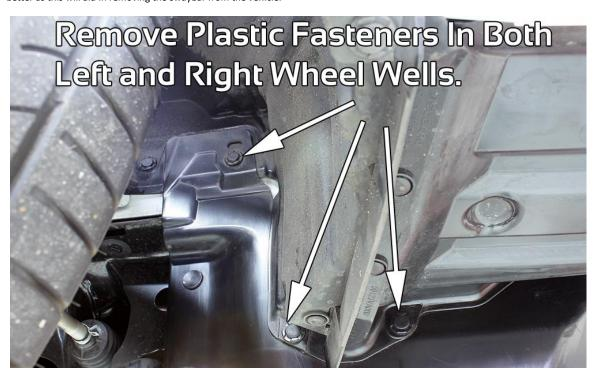
2. Using a panel removal tool or large flat head screwdriver, locate and remove plastic fasteners in each wheel well as shown above. Under the car, locate and remove (3) M8 bolts that secure plastic splash guard to chassis. As the last bolt is removed, push the splash guard to the rear of the car to unclip (2) large plastic clips securing splash guard to chassis.
