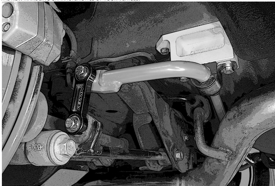
Complete sway bar, Stout Mounts, and endlinks installed
