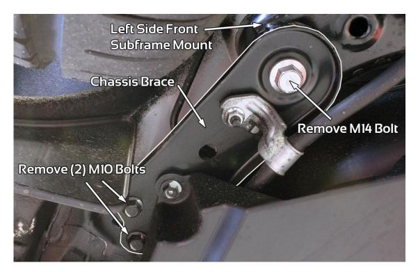
8. Locate both front subframe M14 bolts and (2) braces that secure it to the chassis. Remove (2) M14 bolts securing subframe to the chassis and (4) M10 bolts securing braces to the chassis. Depending on the year of car, the brace will also fall off the car. **NOTE: Some models have a brake cable and/or a plastic guard bolted to each brace. These will hold the brace in place during this step.**
