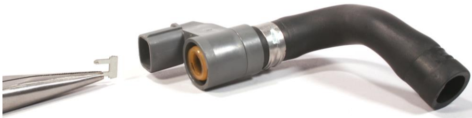
Diagnosis connector shown with jumper pin being pulled out. Plug may be gray or white depending on year of car.
