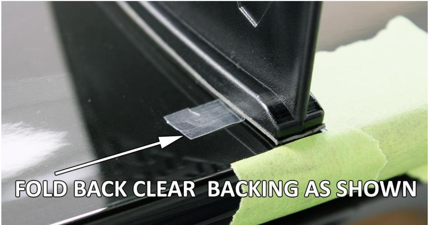
10. While holding wing stabilizer in place, slowly pull clear tape backing from lower portion of stabilizer. This will expose foam tape to trunk, starting the process of adhesion. **Note: This step can be tricky, but pulling tape toward front of car versus straight to the left or right will make this job a little easier.**
