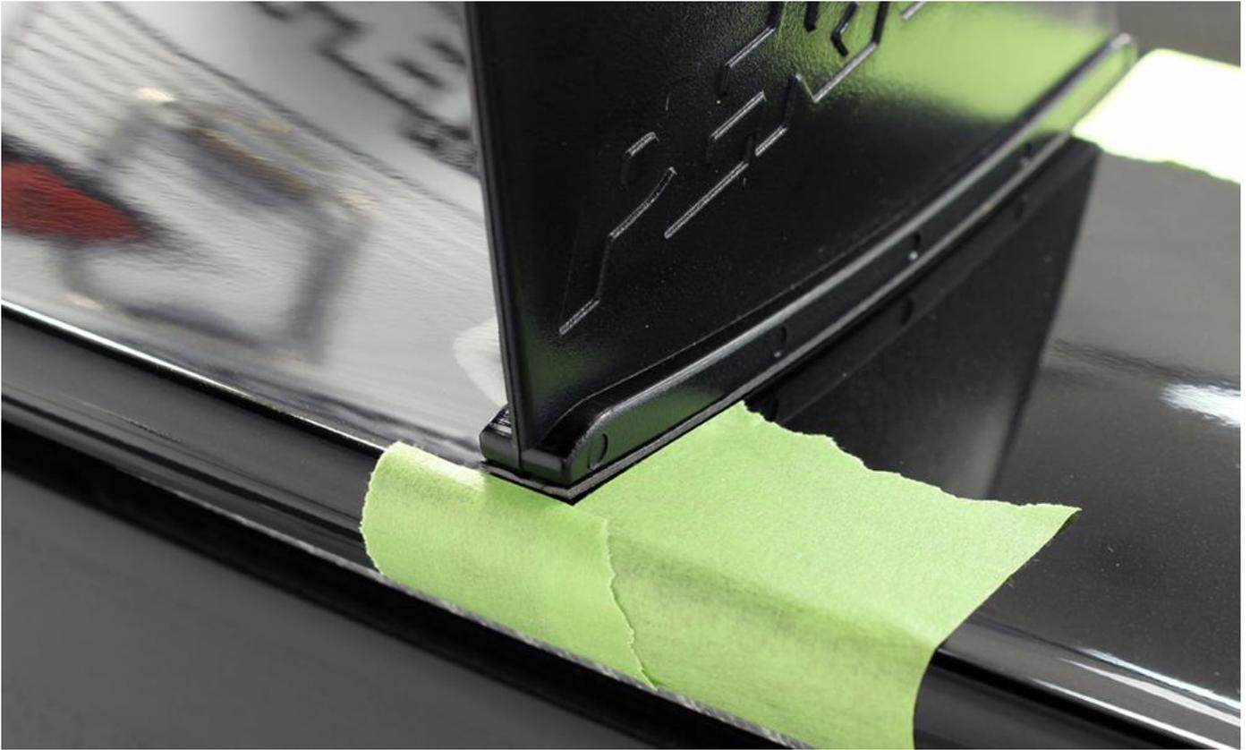
4. Use masking tape or similar to accurately mark location on both under side of wing as well as on trunk as shown. This is done as a guide for final installation. See above picture.
