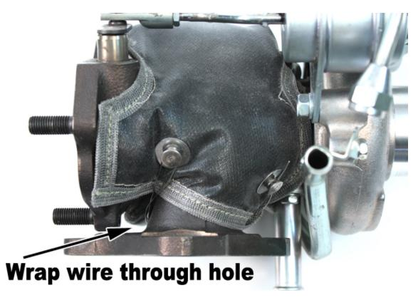
NOTE: Above picture shows a typical WRX or Legacy GT turbo, where wire needs to be routed through hole in front of downpipe flange.
