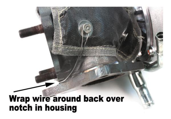
NOTE: Above picture shows a typical STI or aftermarket turbo, where wire needs to be routed below sealing flange and away from uppipe stud. If installing heat blanket with downpipe installed, take care not to wrap wire around downpipe or bolts securing downpipe.
