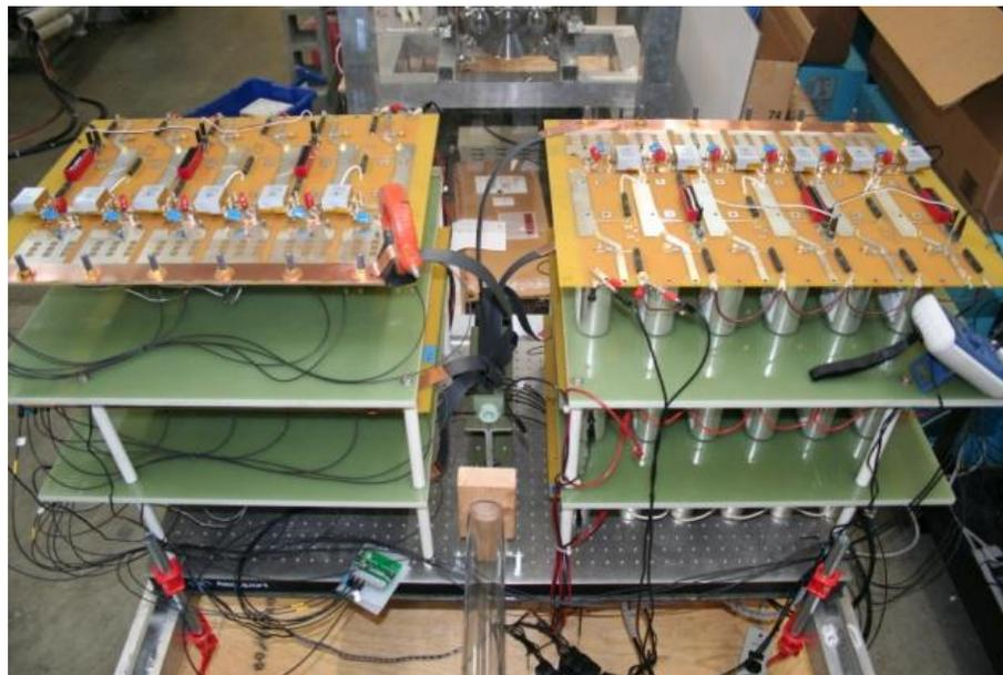
Figure 16 Six stage macron launcher. Shown are solid-state switching, parallel capacitors, fiber-optic trigger and DAQ, and macron launcher.
