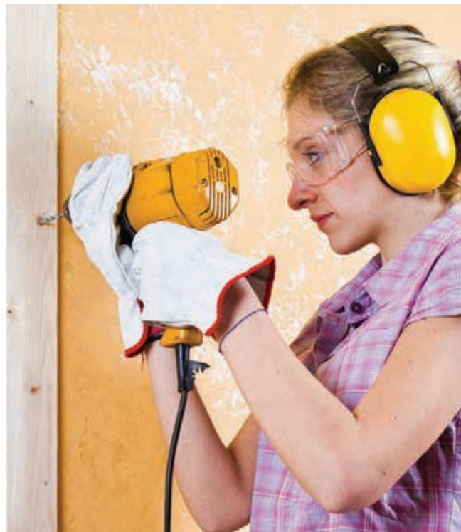
Figure 2-9. When using power tools, be sure to wear appropriate protective gear, such as gloves, safety glasses, and hearing protection.
