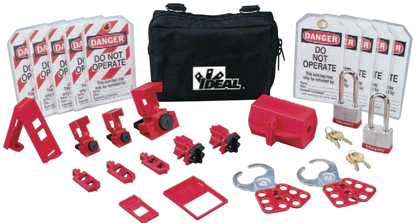
Figure 2-14. Lockout/tagout kits contain various types of lockout devices and tagout devices. Some lockout devices can accommodate multiple locks. This type of device is used when more than one electrician is working on a circuit.
