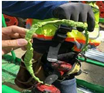
Tool lanyard in use by worker on aerial lift.
