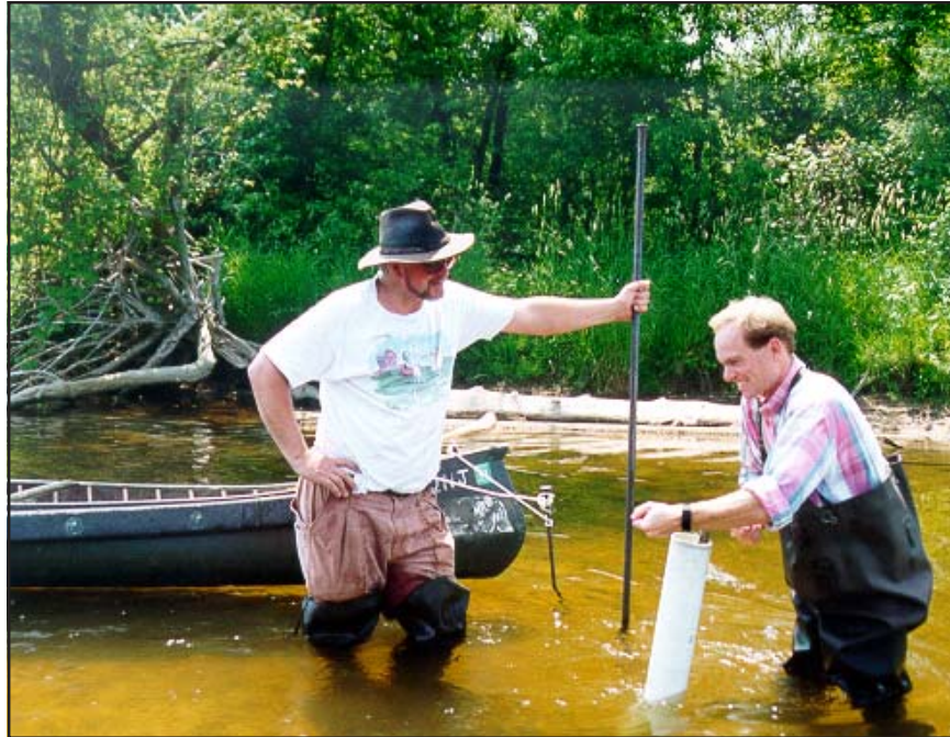
Geologists verified the ground-penetrating radar's readings by coring through the bottom sediments and comparing results.
