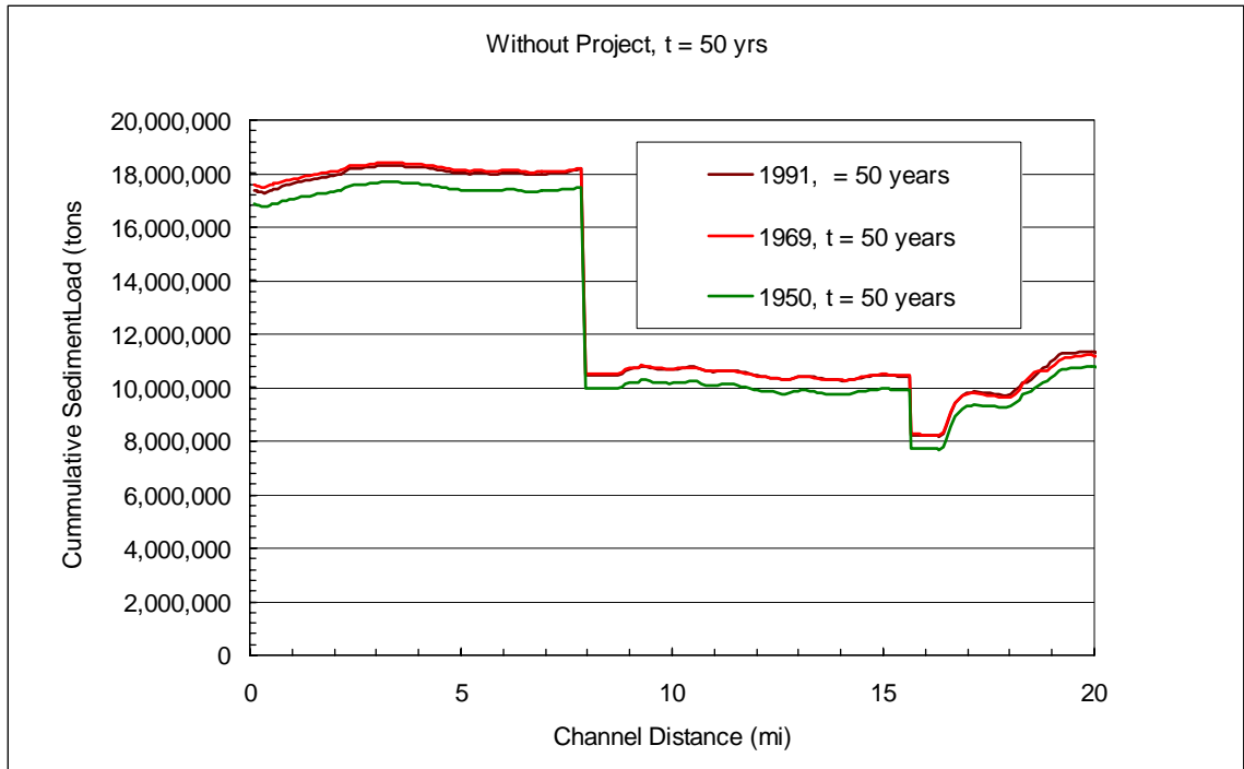
Figure 11.13. Cumulative Sediment Loads at end of 50 year Simulation for Without-Project Conditions for different hydrographs.
