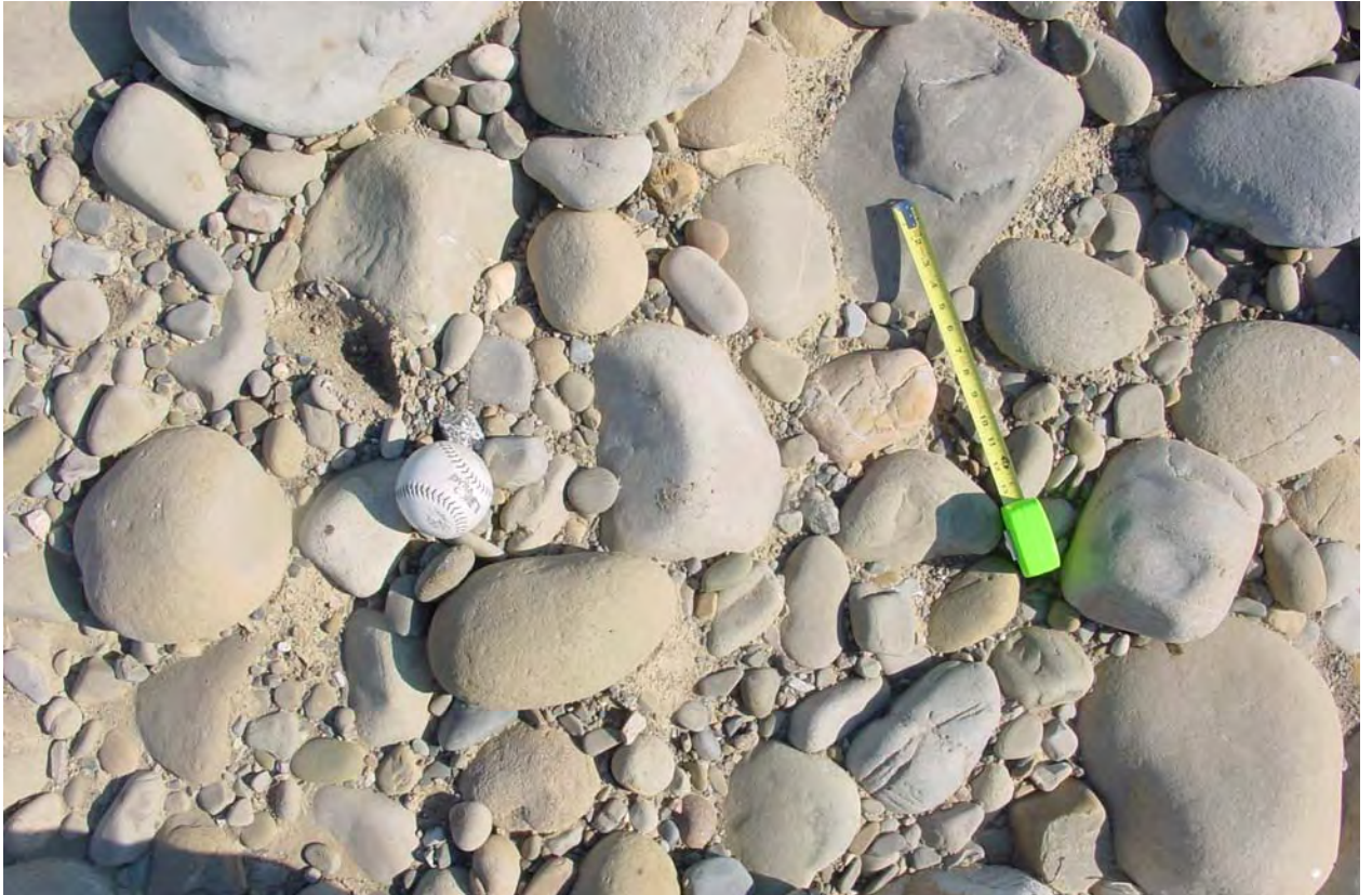
Figure 5.3. Typical Surface Bed Material in Ventura River. Note Large Range of Sizes. A Softball and Tape Measure are shown in Figure for Scale.
