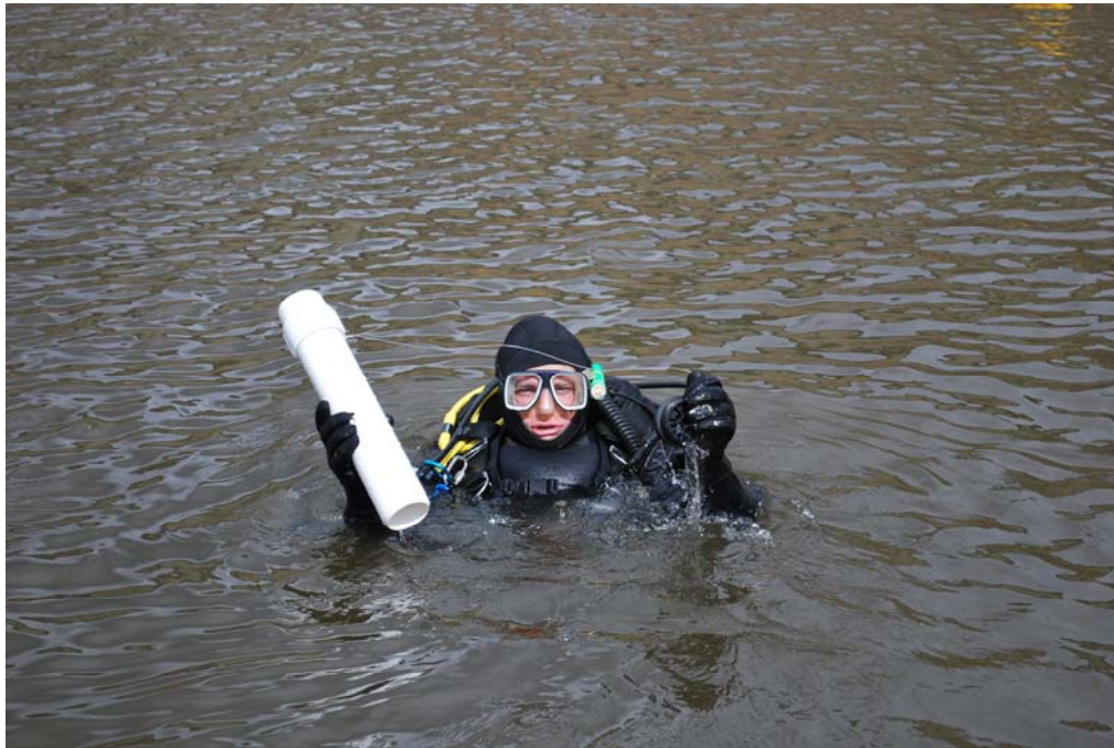
Photograph No. 3 Diver with sediment sampling tube in hand preparing to descend for sediment retrieval. Bureau of Reclamation - Pacific Northwest Underwater Inspection Team. JC Boyle, Copco 1 and Iron Gate Dam, Klamath Hydroelectric Project, Oregon-California – April 12-16, 2010.
