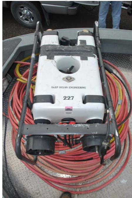
Photograph No. 5 PN Dive team Deep Ocean Engineering ROV. Bureau of Reclamation - Pacific Northwest Underwater Inspection Team. JC Boyle, Copco 1 and Iron Gate Dam, Klamath Hydroelectric Project, Oregon-California – April 12-16, 2010.
