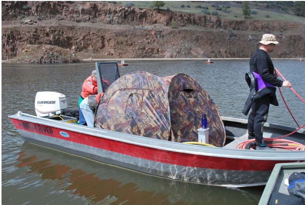
Photograph No. 7 Hunting blind used for viewing ROV video monitor. Bureau of Reclamation - Pacific Northwest Underwater Inspection Team. JC Boyle, Copco 1 and Iron Gate Dam, Klamath Hydroelectric Project, Oregon-California – April 12-16, 2010.
