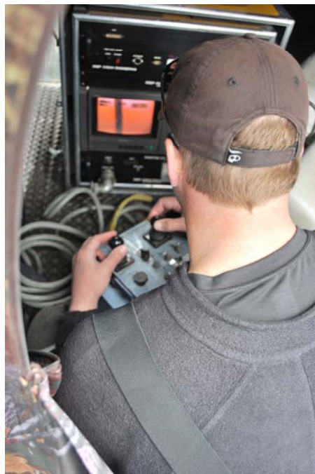
Photograph No. 8 View of ROV controls and video display unit. Bureau of Reclamation - Pacific Northwest Underwater Inspection Team. JC Boyle, Copco 1 and Iron Gate Dam, Klamath Hydroelectric Project, Oregon-California – April 12-16, 2010.
