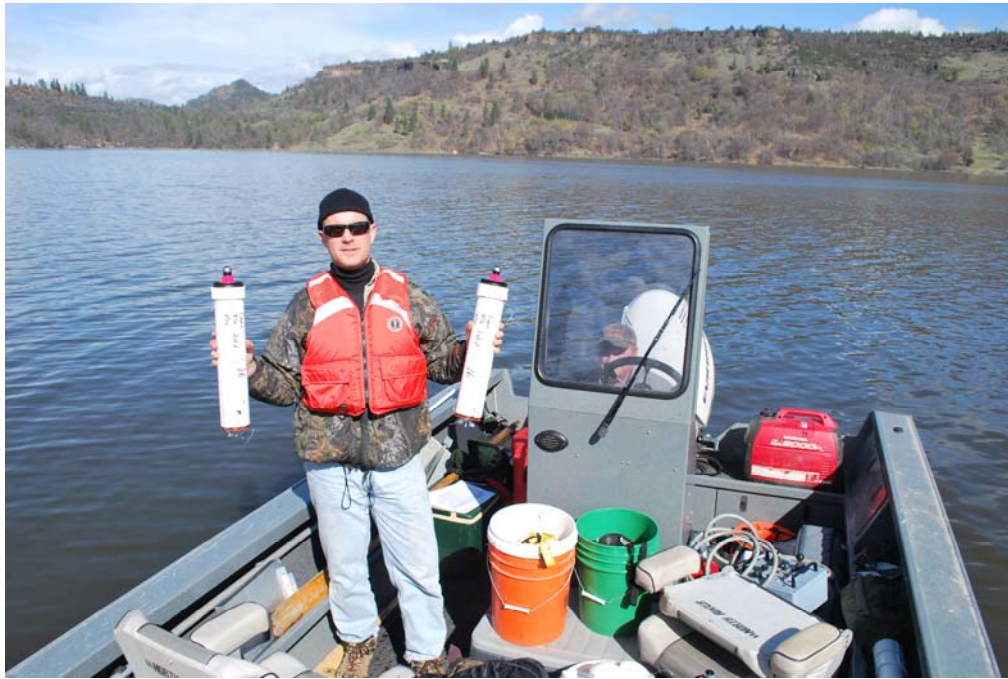
Photograph No. 1 Paul Zedonis (USFWS) showing arrangement and orientation required for proper delivery of sediment sampling tubes to the surface. Bureau of Reclamation - Pacific Northwest Underwater Inspection Team. JC Boyle, Copco 1 and Iron Gate Dam, Klamath Hydroelectric Project, Oregon-California – April 12-16, 2010.
