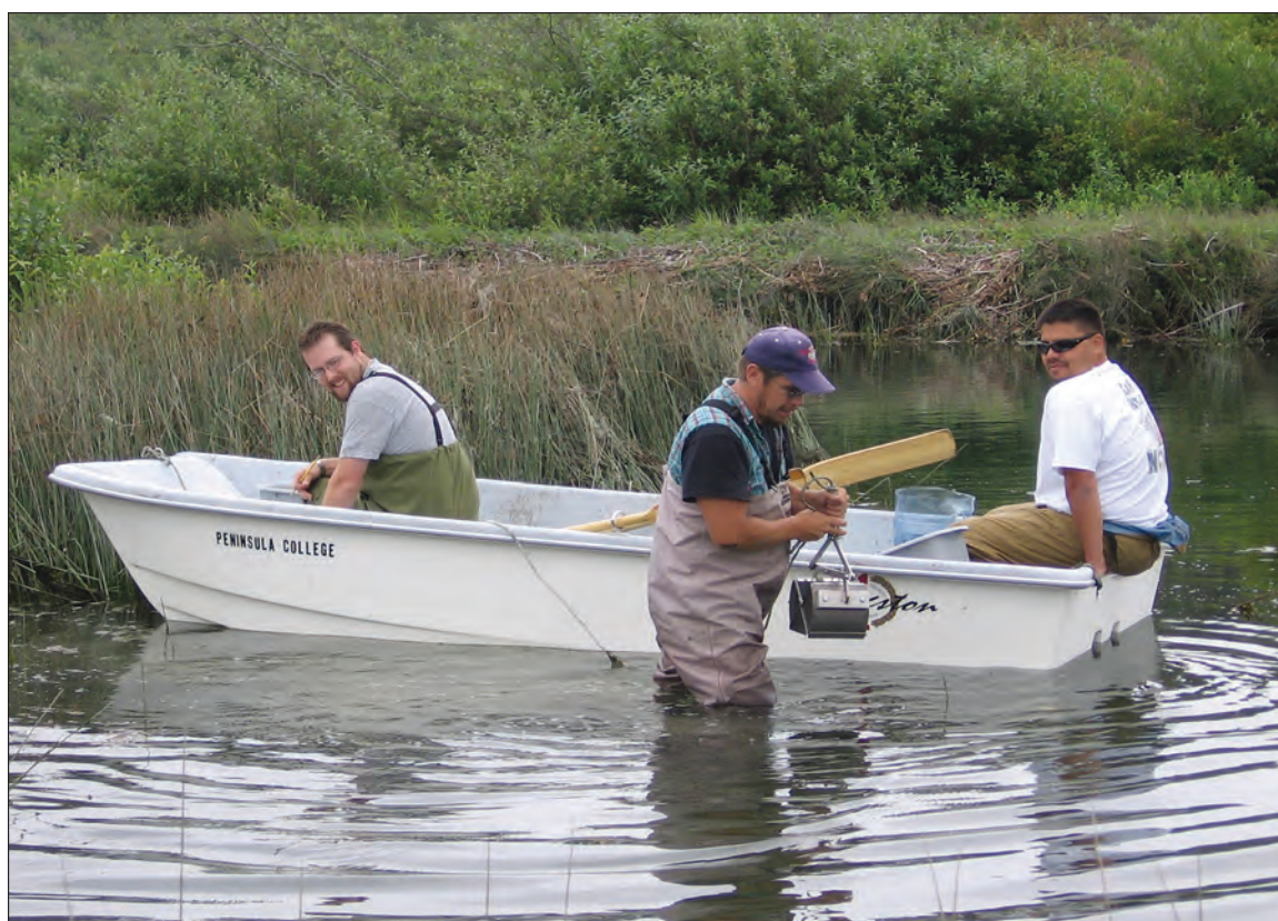
Figure 7.3. Lower Elwha Klallam Tribe fisheries technicians sampling sediments in the Elwha River, Washington, estuary using a petite Ponar grab sampler. (Photograph taken by Matt Beirne, Lower Elwha Klallam Tribe, April 17, 2006.)
