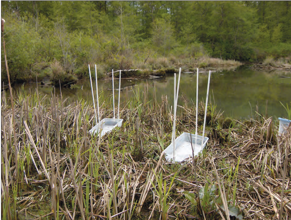
Figure 7.7. Two flight-intercept (fallout) traps placed in littoral habitat of the Elwha River estuary, Washington. Each trap is attached with rings to PVC stakes, allowing the trap to rise and fall during tidal fluctuations. (Photograph taken by Matthew M. Beirne, Lower Elwha Klallam Tribe, April 26, 2006.)
