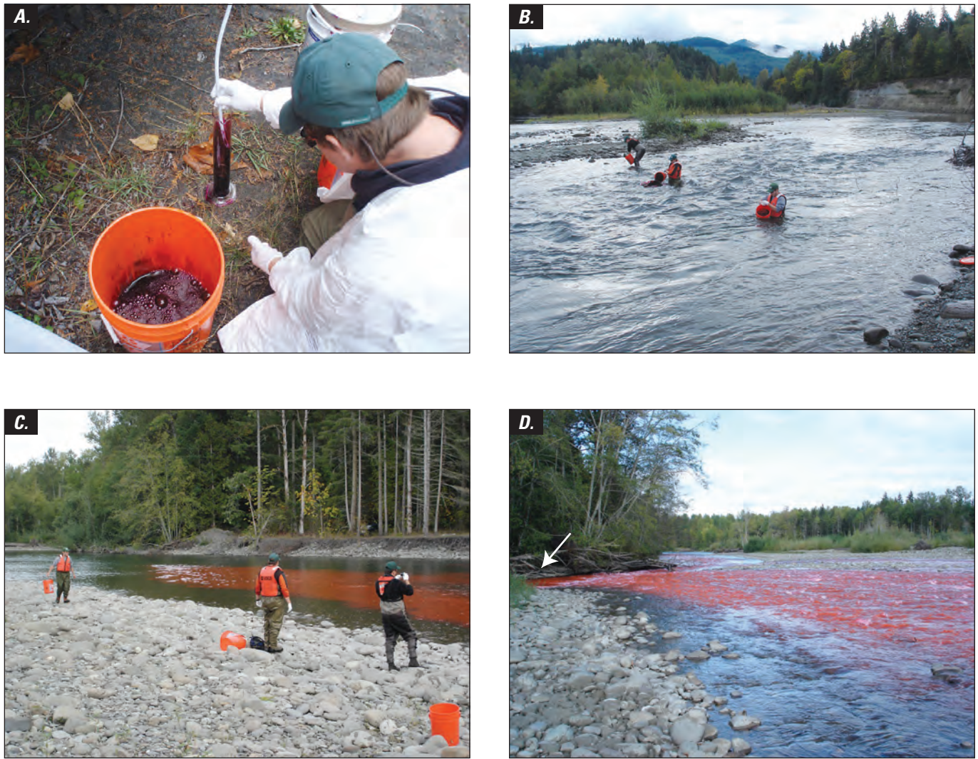
Figure 4.5. Dye study in the lower Elwha River, Washington, September 29, 2009. (A) USGS hydrologist mixing the Rhodamine WT solution prior to slug injection; (B) three USGS hydrologists introducing the rhodamine into a riffle to enhance lateral mixing of the tracer; (C) dye tracer just downstream of the injection riffle, where the plume is spreading longitudinally and laterally in the slow moving water before reaching the next downstream riffle; and (D) looking downstream as the dye tracer approaches the first monitoring station. Main channel storage is evident on the left side of the channel in a slower moving backwater area, shown by the arrow. (Photographs taken by (A) James R. Foreman, U.S. Geological Survey and (B, C, D) Christopher A. Curran, U.S. Geological Survey.)
