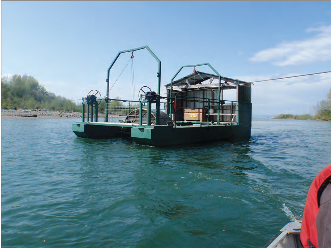
Figure 7.11. A 2.5 meter rotary screw trap operated at river kilometer 0.5 by the Lower Elwha Klallam Tribe fisheries office for counting juvenile salmon emigrating from the Elwha River, Washington. (Photograph taken by Michael L. McHenry, Lower Elwha Klallam Tribe, May 26, 2010.)
