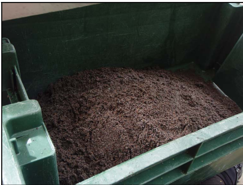
Figure 3-14. Bedload sample collected at 5,000 cfs on May 15, 2008 (#2008-20).
