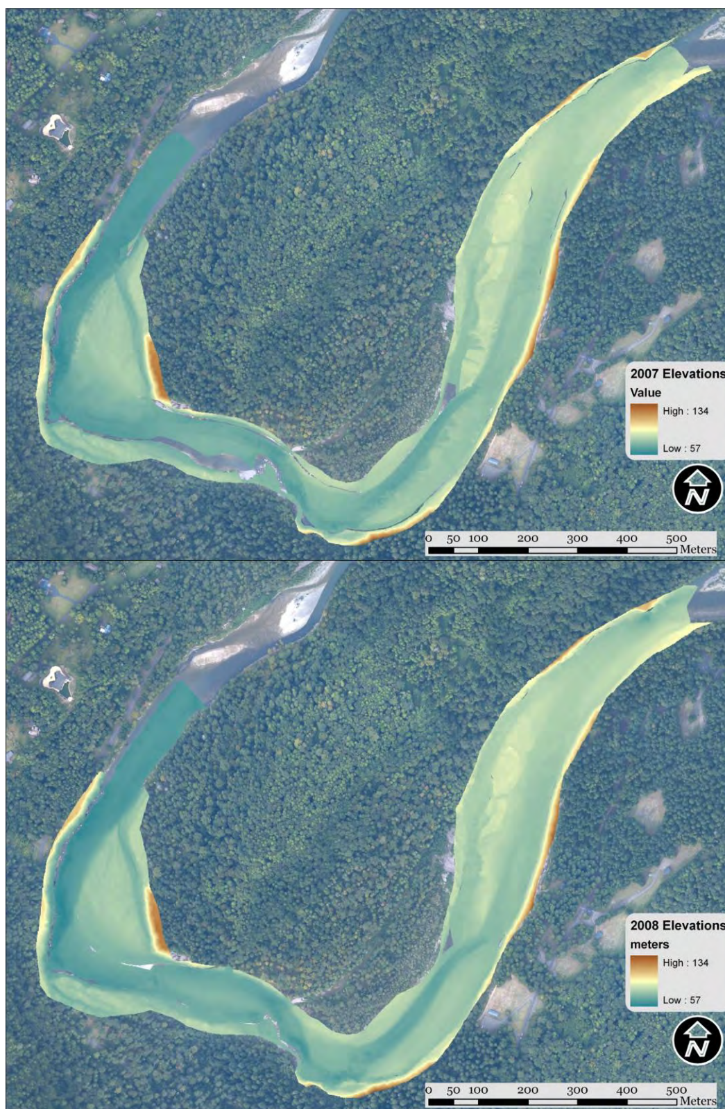
Figure 16 - DEM generated from survey & LiDAR for Oxbow Reach (2007 on top, 2008 on bottom)
