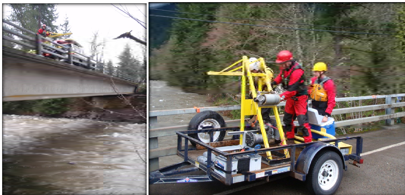
Figure 21 - Bridge Crane Sampling Setup
