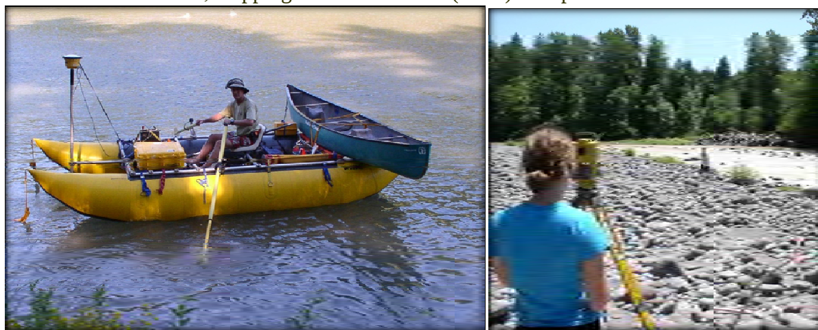
Figure 12 - Surveying Setups. Cataraft (left) with GPS antenna mounted on the mast. Total station (right).
