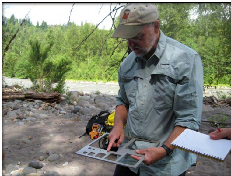
Figure 20 - Gravelometer (demonstrated by Dr. Peter Wilcock, JHU)
