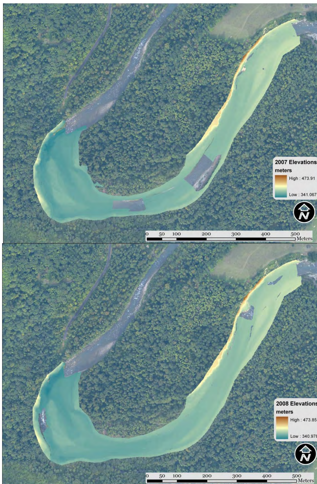
Figure 15 - DEM generated from survey & LiDAR for Cedar Creek Reach (2007 on top, 2008 on bottom)
