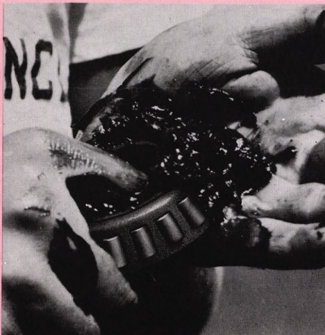
Fig. 8 Greasing a roller bearing.
