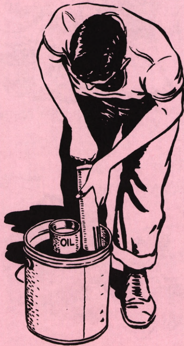
Fig. 7 How to fill a grease gun.
