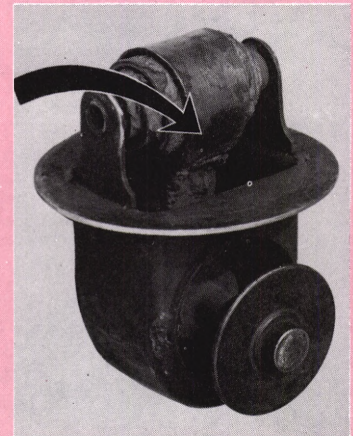
Fig. 6 A metal strip thermostat that has been ruined by scale.
