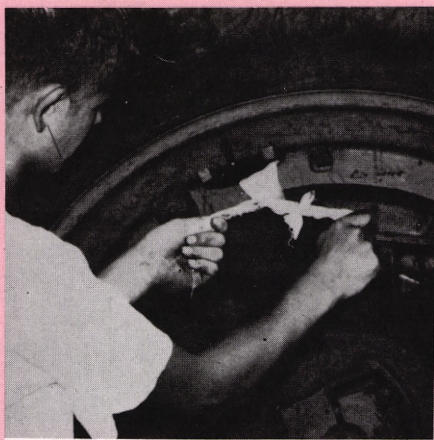
Fig. 11 Check slippage by tying a cloth to a spoke and counting off 30 revolutions.
