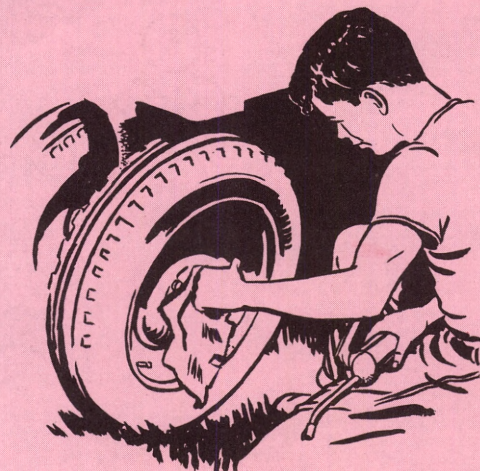
Fig. 4 Wipe fittings before greasing.
