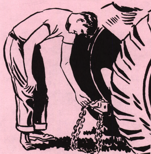
Fig. 18 Ground your tractor when doing belt work.
