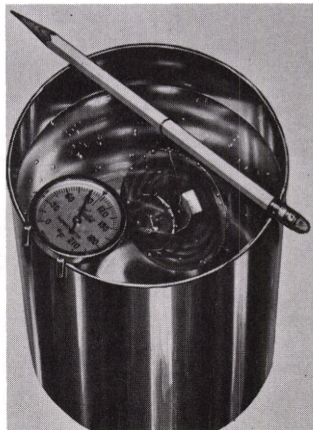
Fig. 8 Checking a new thermostat.
