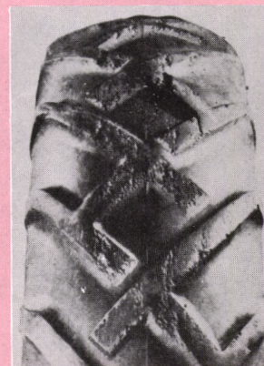
Fig. 7 Excessive slippage causes tread wear.
