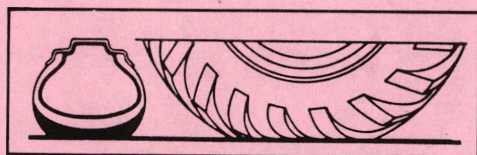
Fig. 3 Under-inflation is tough on tire sidewalls.
