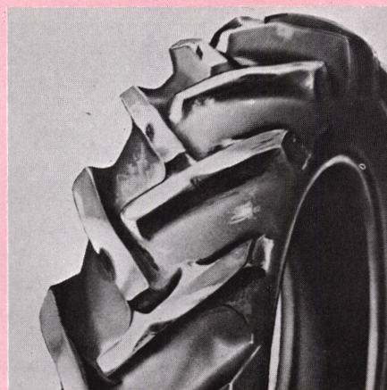
Fig. 15 Irregular wear caused by operating the tire at low pressure on a hard road surface.
