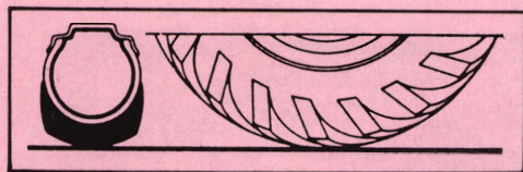
Fig. 4 Over-inflation can cause rapid tire wear.
