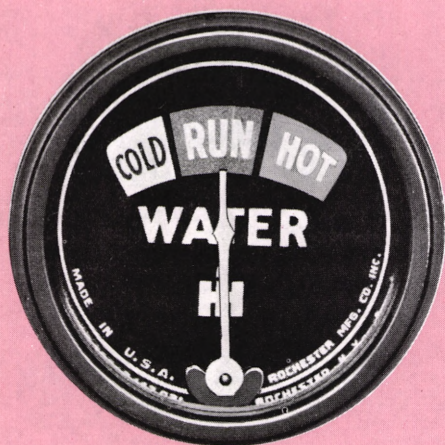
Fig. 2 A cooling system temperature gauge.
