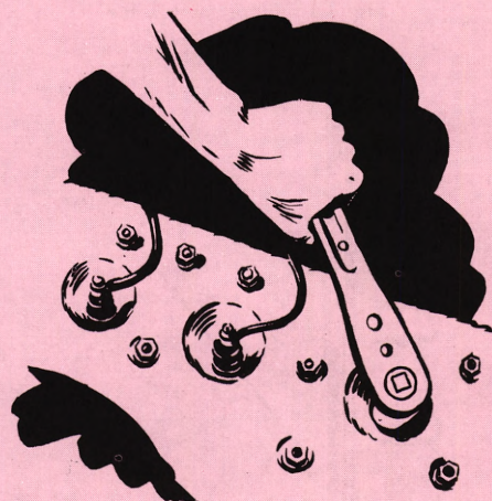
Fig. 15 Use a socket wrench on spark plugs.
