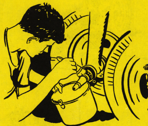
Fig. 17 Cleaning a bearing that stays on the axle.
