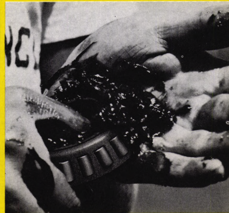
Fig. 16 How to pack a bearing.
