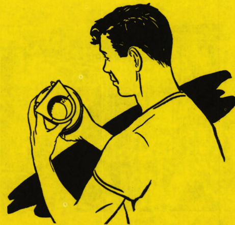
Fig. 20 Check the muffler for restrictions, dirt, etc.
