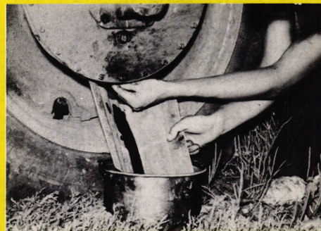
Fig. 24 A metal trough keeps gear lubricant off the tires.
