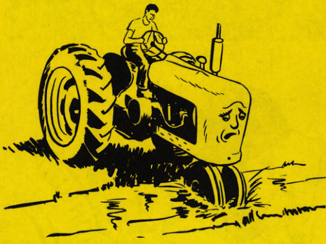
Fig. 12 If you get your front wheels wet—re-lubricate.
