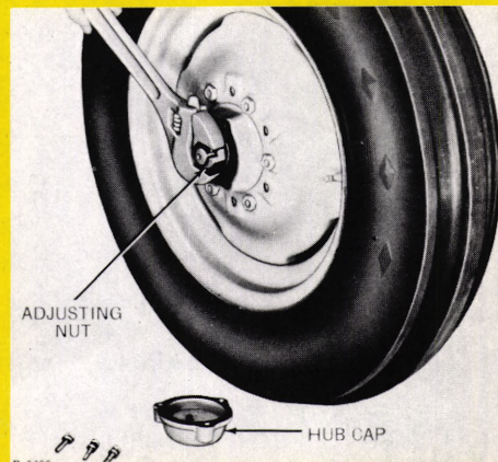
Fig. 19 Tightening a front-wheel bearing. Is this wrench being used correctly?
