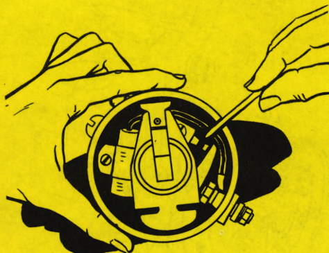
Fig. 11 Rotating the distributor case to time a battery ignition engine.
