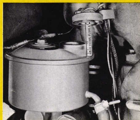
Fig. 6 A tractor that has its own power steering oil supply.
