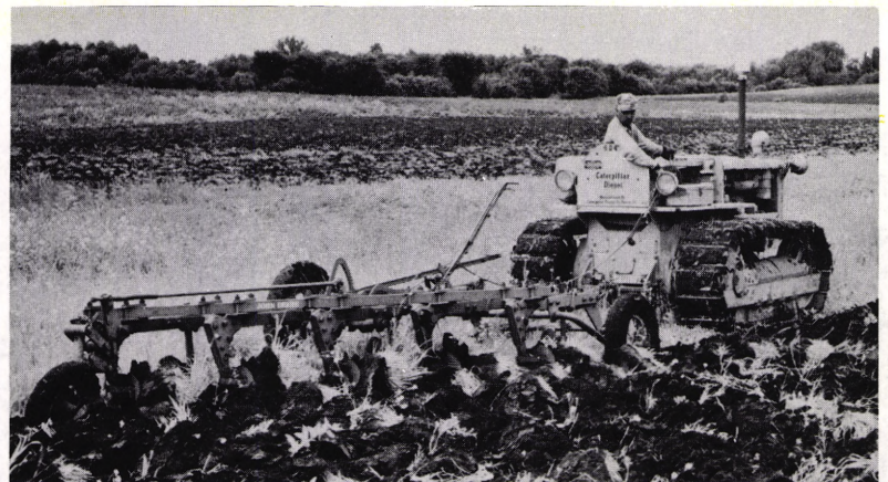
Fig. 4 Your engine governor keeps the tractor moving at constant speed.
