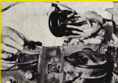
Fig. 10 Checking direction in which rotor turns.
