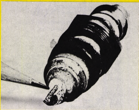
Fig. 21 Broken spark plug porcelain.
