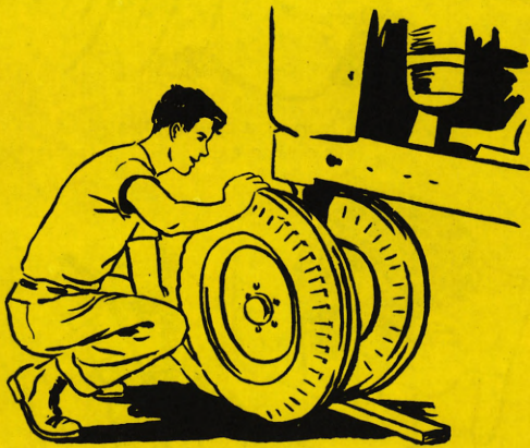
Fig. 13 Checking a front wheel for play.
