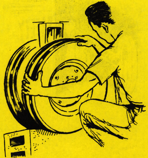
Fig. 13 Checking for loose steering. Is your tractor safe?
