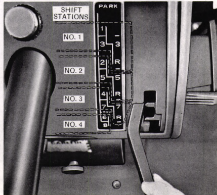
Fig. 8 Modern tractors have a wide selection of gears.
