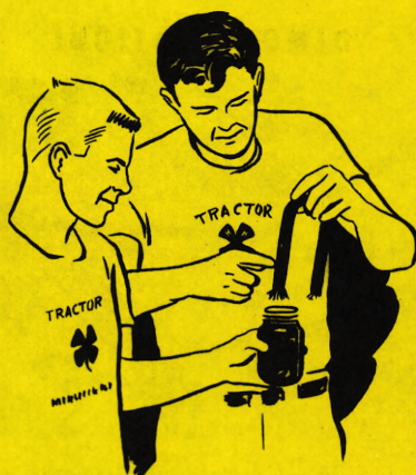
Fig. 20 Using a magnet is a good test for metal particles in your gear lubricant.
