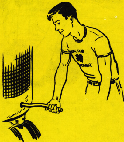
Fig. 3 Checking compression by cranking the engine.
