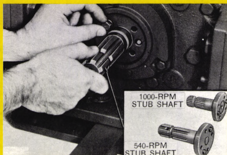
Fig. 11 Changing the stub shaft to change the PTO speed.
