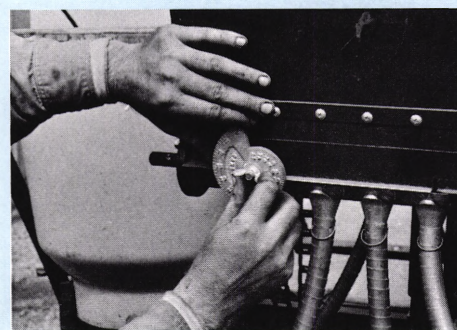
Fig. 17 Set the dial indicator for the desired application rate.
