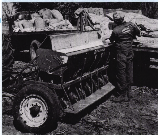
Fig. 18 Keep the fertilizer attachment cleaned out.
