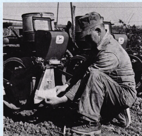
Fig. 18 Make a calibration run in the field, collecting the granules for a known acreage.
