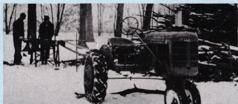
Fig. 1 Tractor power can be used to drive belts.
