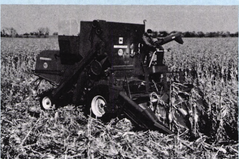
Fig. 20 Corn combine picks the ears and shells the corn.
