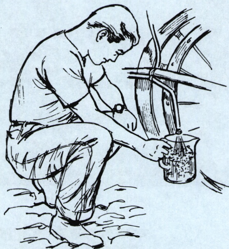
Fig. 12 Checking nozzle discharge rate.
