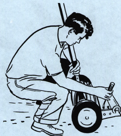
Fig. 11 How to adjust the shear bar on your lawn mower.
