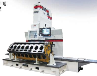
**EM105H** Multi Purpose CNC Machining Center for Medium to Large Blocks
