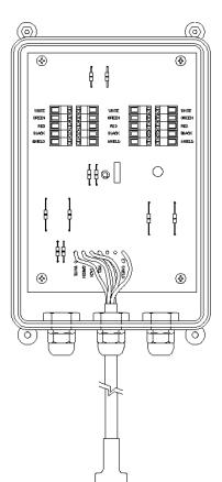
To connect the load cells, attach the junction box cable to the J902 connector on the bottom panel of the scale. Connect the load cell cables to the junction box as shown left.
