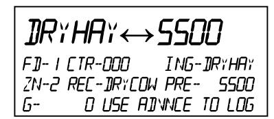
The upper display will flash between the ingredient name and the call weight:
