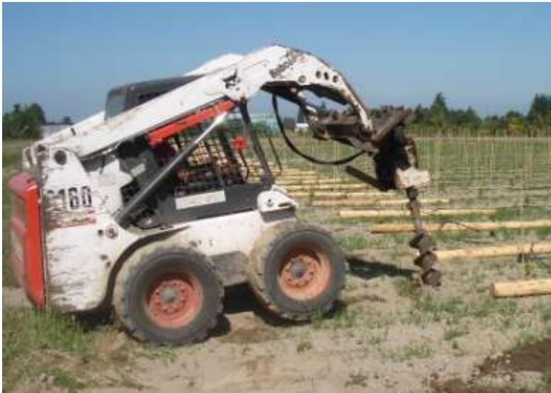
**Figure 1.** Drilling postholes for end posts
