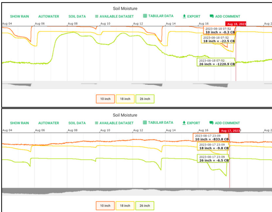
Figure 3. Soil water availability measured by tensiometers at 3 depths in soil profile under SD (top) and DRZ (bottom) drip irrigation. Water tension expressed in negative centibars.
