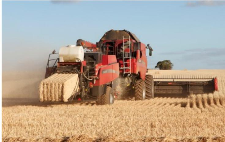
Figure 3. Bale direct system operating during wheat harvest in Australia.
