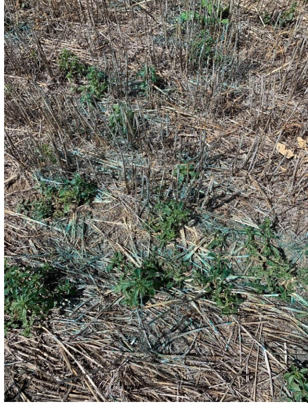
Figure 1 (above). Weeds sprayed with weed sensing sprayer system. Blue dye was added to the application solution to check system efficacy.
