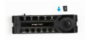
Insert the microSD Card into the card slot on the Controller.
