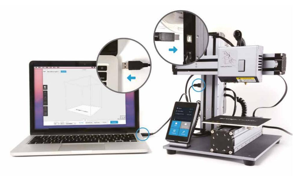
Connect the computer to the machine using the provided USB Cable.
