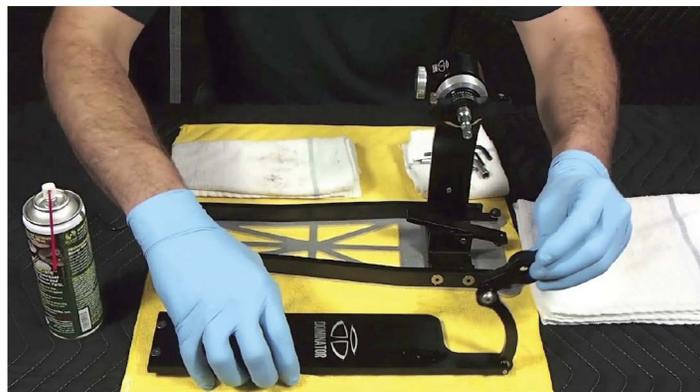
**Lubricating footboard, hinge, and heel plate.**
