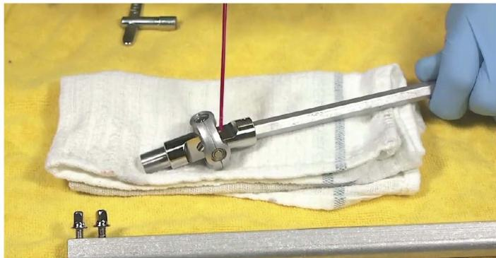
**Lubricating u-joints for smooth, vibration-free response.**
