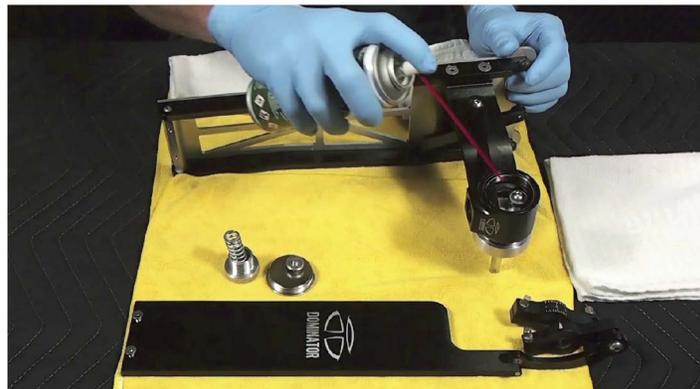
**Applying barrier film lubricant to all moving metal parts.**
