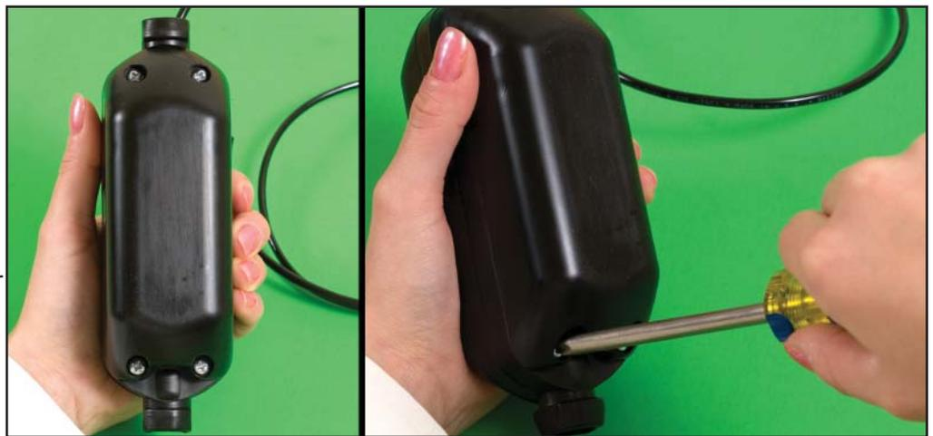
2. Once all four screws have been removed, lift the battery module straight off of the electronics module. Do not twist either module; doing so may damage the electrical connectors between the modules.
