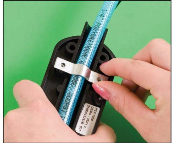
5. Install the first hose clamp using the 6-32 x 1/4" Phillips pan head SEMS screws. Use a #2 Phillips screwdriver to tighten the screws. Tighten snugly, do not overtorque, and do not bend the clamps. Finish this step by installing the second hose clamp of the same size at the second hose clamp position.
