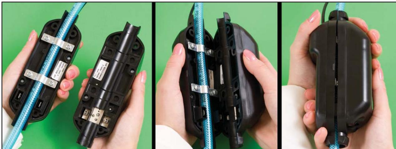
7. Secure the battery module in place against the electronics module using either or both of the two types of securement provided.
