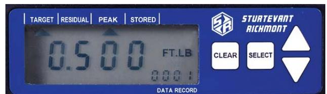
The large number in the center is the Target, or the midpoint value between the minimum and maximum (Lo and Hi) torque values currently active on the tool. The active Target arrow verifies this.
