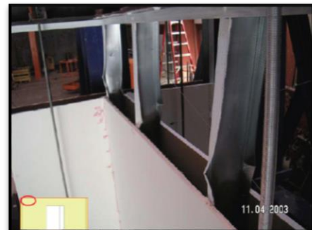
Figure 4. Buckling of studs for a fixed connection partition wall
