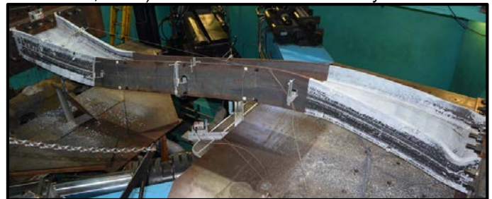
Figure 13. Failure modes of steel columns (Uang, Ozkula and Harris, 2015). W24x176 with P = 0.18P_y .
