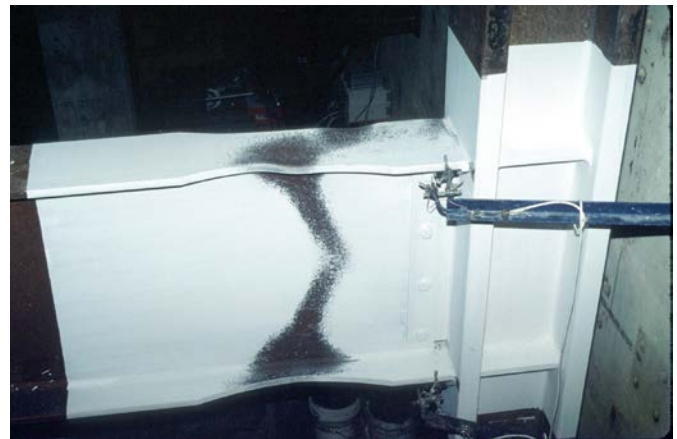
Figure 10. Test data for a post-Northridge reduced beam section ductile connection (Engelhardt and Sabelli, 2007)
