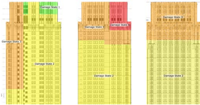
Figure 8. Image of damage predictions for historic façade using FEMA P-58; this was done as a part of a comprehensive risk assessment of this building, in support of a purchase decision.
