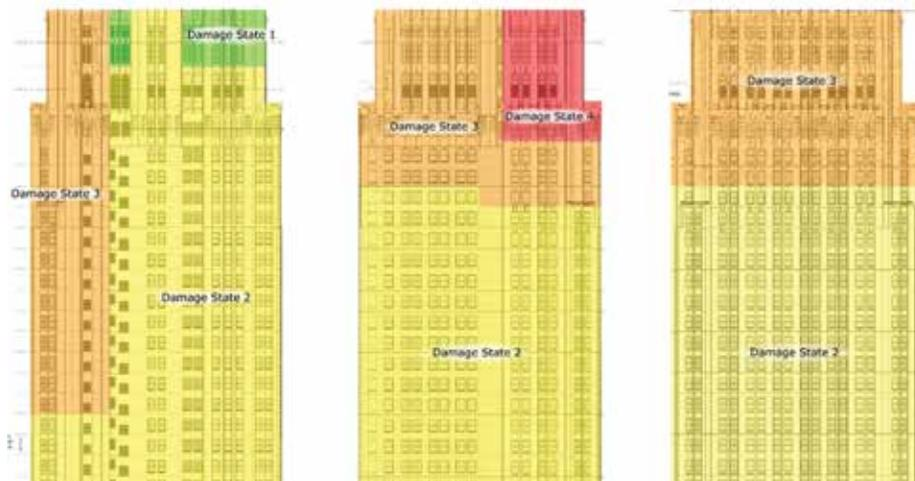
Figure 8. Image of damage predictions for historic façade using FEMA P-58, done as a part of a comprehensive risk assessment of this building, in support of a purchase decision.
