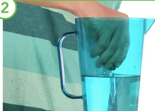
Fill the glass eyedropper about 1/4 full with water. You may need to experiment with the amount of water in the eyedropper in a test cup, as it should be just enough water to make it so the eyedropper is barely floating.
