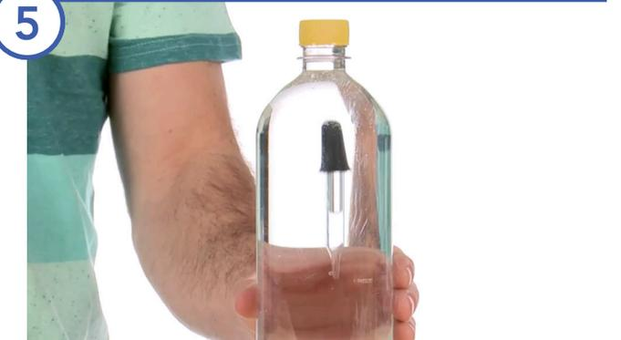
Gently squeeze the sides of the bottle and notice how the eyedropper sinks. Release your squeeze and it floats back up to the top.
