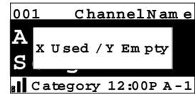
2. By holding down the MEMO button for 3 seconds, the stored memory information (one at a time) is displayed on the LCD screen in page format. Use the Encoder knob to scroll through the 24-page listing and view the information. This function allows you to recall information regarding the Artist/Song Title for your own personal review. To return to the default tuning mode press and hold the MEMO button for 3 seconds.
