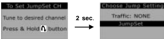
Once the Jump button is set to function as JumpSet, the Traffic line displays "NONE" to signify that the button can no longer be set to traffic alert.
