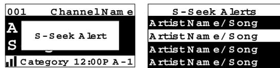
No stored match alert is provided for the currently selected channel. To ensure that no duplicate entries are stored in memory, the receiver will check the stored input data to ensure the information about to be stored is not already in memory.
