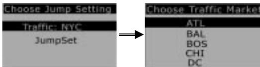
Rotating the encoder knob or pressing the CH+/CH- button on the remote scrolls through the city list, highlighting each city for selection. When the desired city is highlighted, press the Encoder knob to confirm selection. The city ID is then saved for the Jump feature. If the action is canceled without making a selection (by pressing MENU to return to main menu), no city ID is saved. However, if a city is
