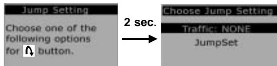
**NOTE:** The Jump button can be programmed to select either of the jump setting options, but not both.
