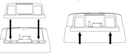
**C.** Once the adapter is seated correctly in the Home Dock, gently press the top of the adapter against the dock with your finger until it clicks into place. The Radio Dock Adapter is now installed.
