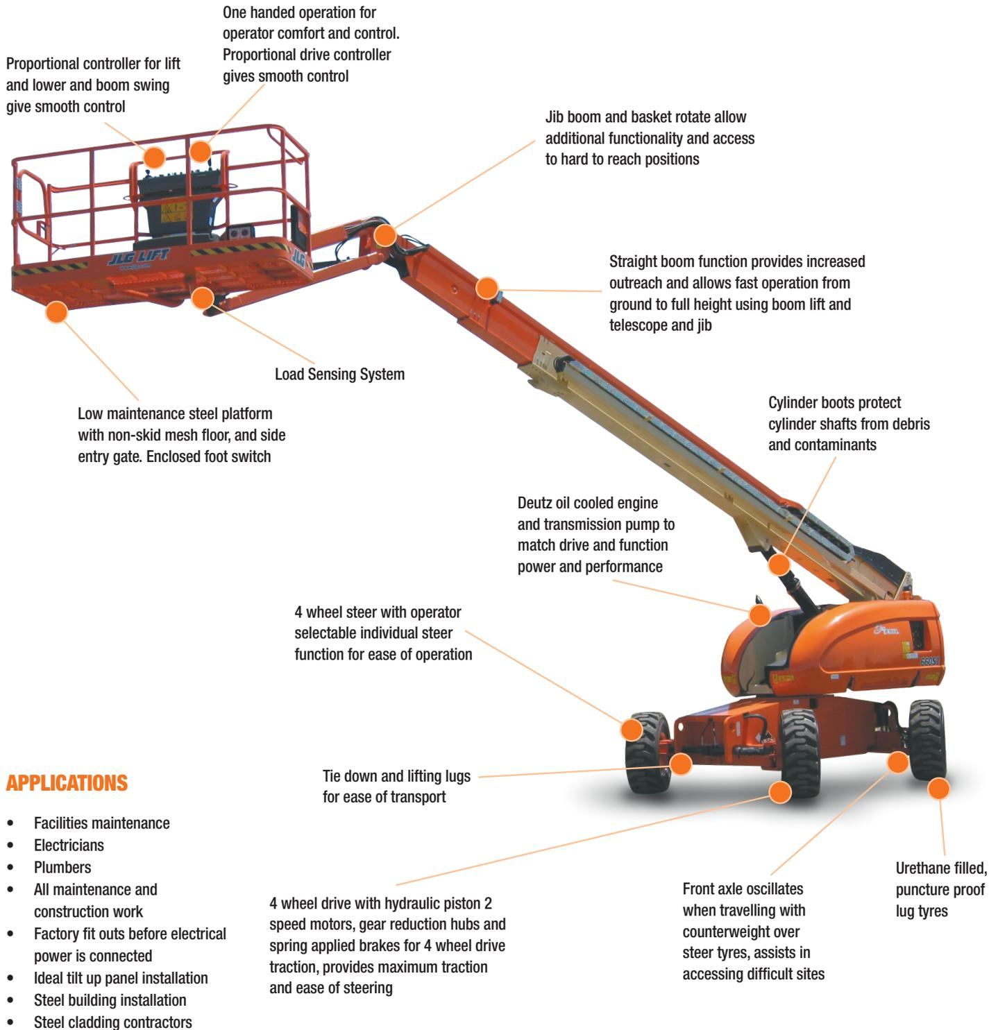
Proportional controller for lift and lower and boom swing give smooth control
