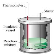
Ideally any calorimeter would be able to completely maintain the system without losing heat to the surroundings. Unfortunately, no calorimeter is perfect and heat is always lost to the surroundings. It is possible to determine how much heat is lost by the calorimeter by mixing hot water and room temperature water. The heat lost by the hot water is equal to the heat gained by the room temperature water.
